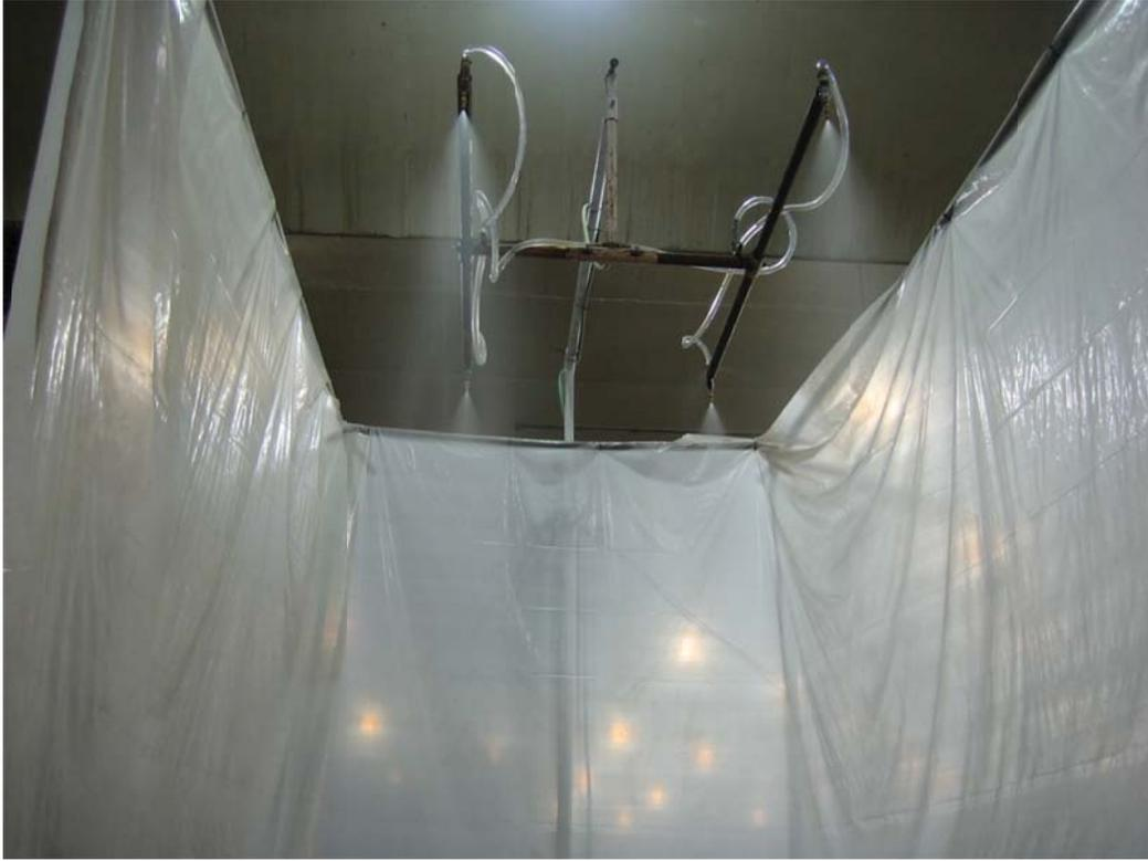
Figure 4. The rainfall simulator with 4 spray nozzles.
