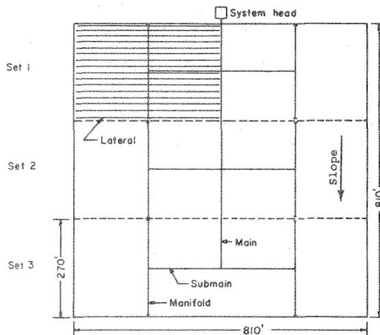
Figure 3: A typical 15-acre (6-hectare) system layout showing various system components.
