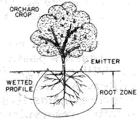
Figure 1: A wetted profile develops in the root zone below each "emitter" or "trickler."
