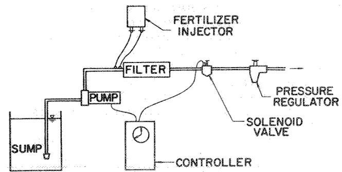
Figure 2: Typical trickle system "head."
